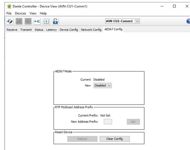
Fig 7-17: AES67 Config tab with AES67 mode disabled
