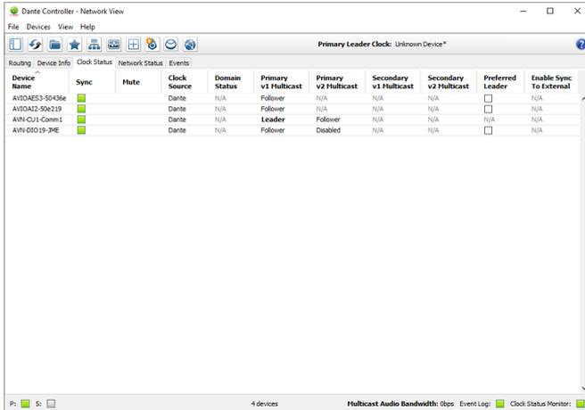
Fig 7-17: Clock Status using and AES67 Master Clock
