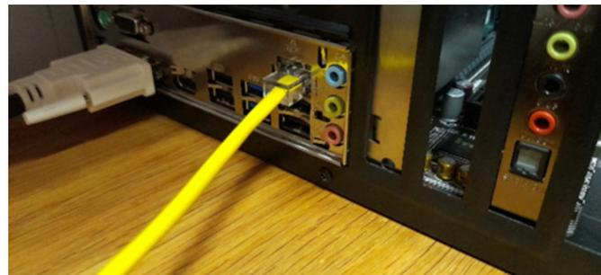
6. Connect an Ethernet cable to an Ethernet port on your PC.
