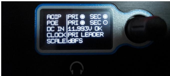
5. When powered using a DC supply, the 'DC IN' field on the display will display the voltage being supplied by this connection and the status of 'OK', e.g. '11.993V OK'. It is possible to power the unit with PoE and DC at the same time for redundancy.
