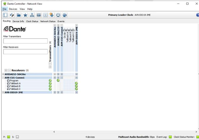
Fig 7-4: Device with default channel labels for AVN-CU1
