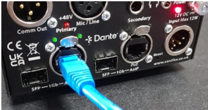
1. Plug an Ethernet cable into the primary port of the AVN-CU1.
