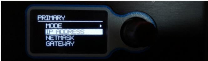
11. Select the 'IP Address' field and enter an IP address which is within the same subnet of your PC. In this case the PC's IP Address is 169.254.228.190 so the IP address 169.254.228.191 was entered. As the subnet mask in this case is 255.255.0.0, the device can be given any valid IP address as long as it starts with 169.254.
