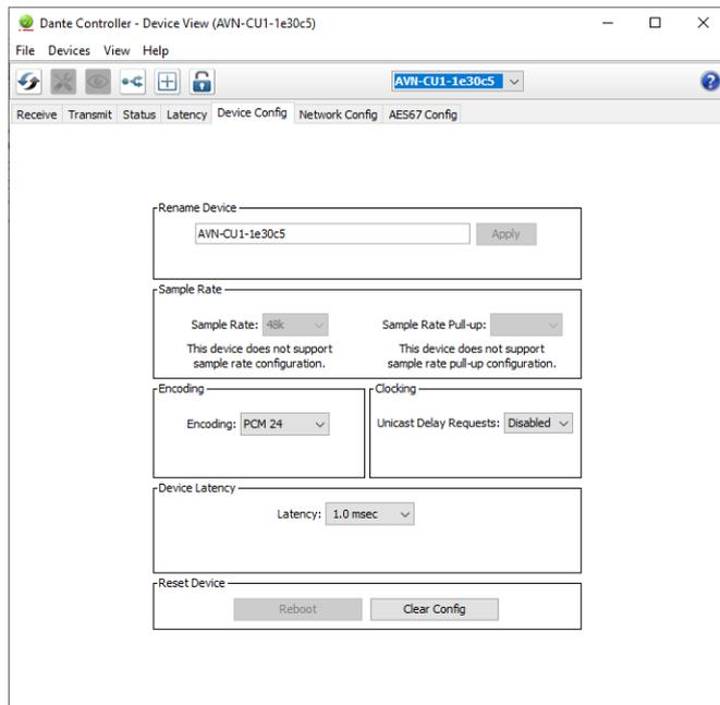
Fig 7-2: Device Config Tab
