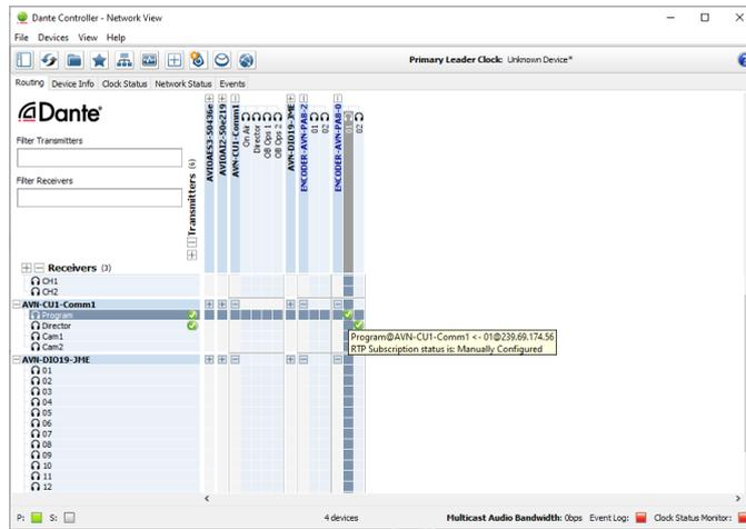
Fig 7-13: Receiving audio from an AES67 device
