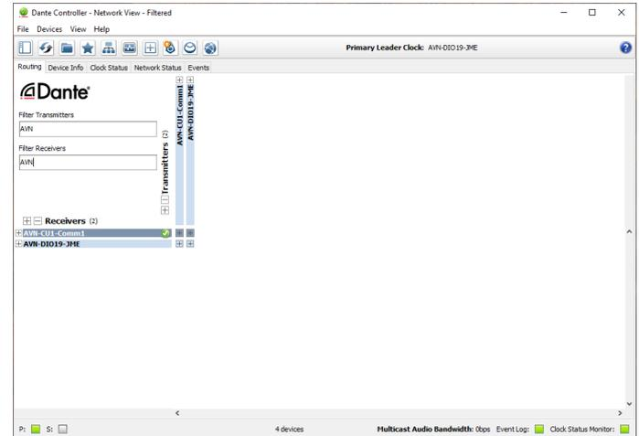
Fig 7-9: Filtering transmitters and receivers
