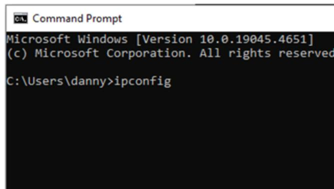
8. In order to find the IP address of your Windows computer open the start menu and type 'Command Prompt', open Command Prompt and type 'ipconfig'. And then press enter.
