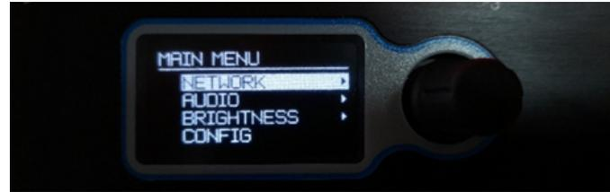
10. Press the encoder for around 1 second to bring up the 'Main Menu' of the AVN-CU1. Press again to enter the 'Network' menu and again for the 'Primary' menu.
