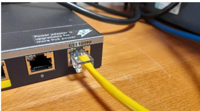
7. Connect the other end of this Ethernet cable to your network switch.
